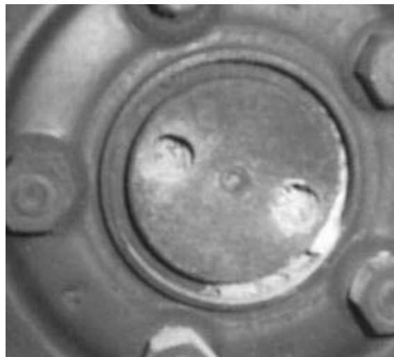
Shown above is a 31 spline shaft end in a 69 Cyclone CJ
